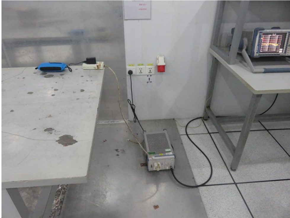
Photo of Conducted Emission Measurement
