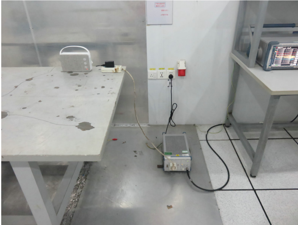
Photo of Conducted Emission Measurement
