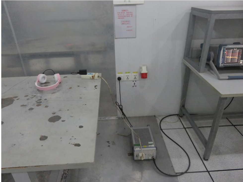
Photo of Conducted Emission Measurement
