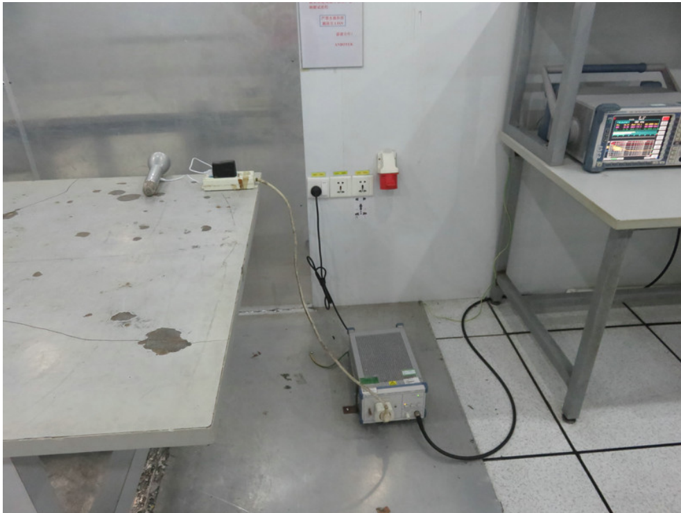
Photo of Conducted Emission Measurement
