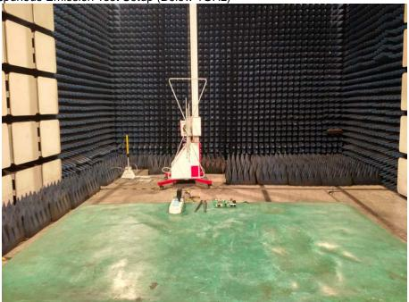
Spurious Emission Test Setup (Below 1GHz)
