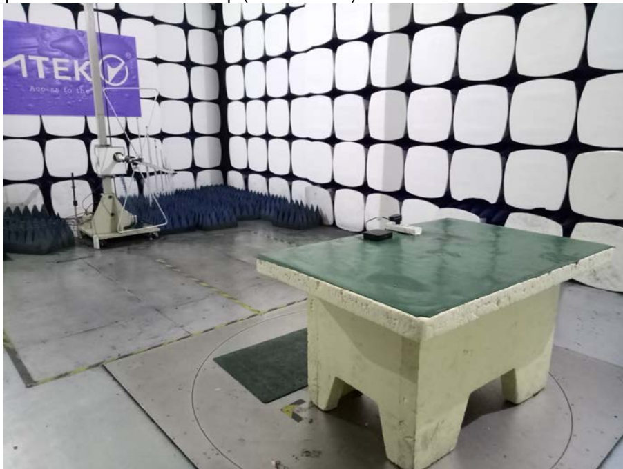
Spurious Emission Test Setup (Below 1GHz)
