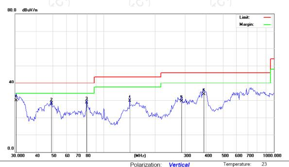
Limit: FCC Part 15B Class B RE\_3 m Power: AC 120V/60Hz Humidity: 54 %
