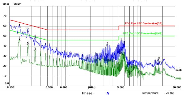
Site Phase: N Temperature: 25 (C Limit: FCC Part 15C Conduction(QP) Power: AC120/60Hz Humidity: 55 %RH
