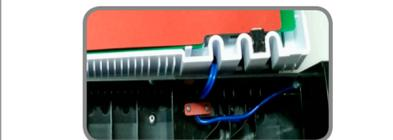
**Make sure to put the wires through the grooves.**
