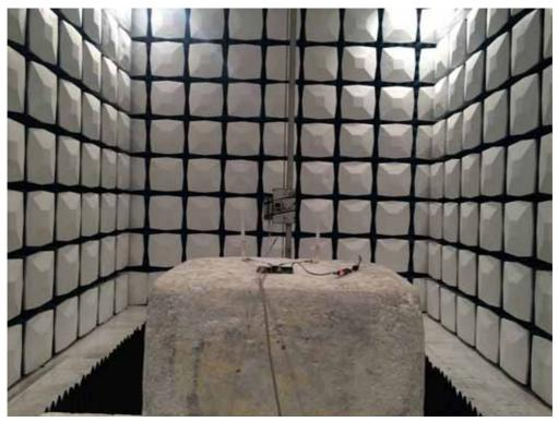
Description: Radiated Emission Test Setup for 1~18GHz
