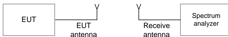
Figure 7.2.1 Carrier frequency separation test setup
