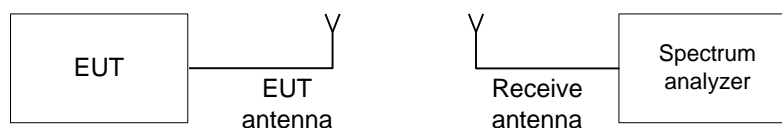
Figure 7.2.1 Carrier frequency separation test setup
