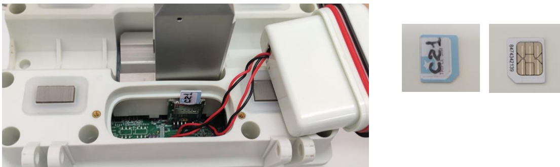
Figure 3: Inserting micro-SIM card into SIM socket
