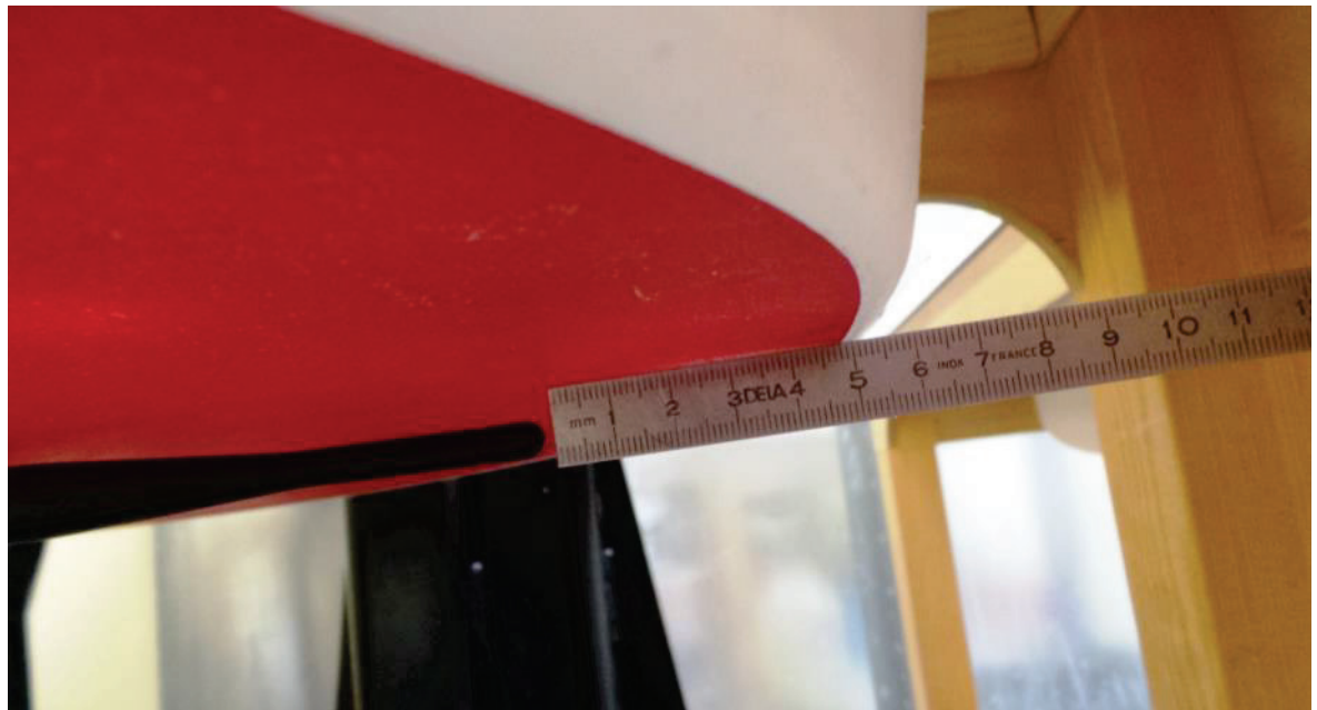
Fig. 12: SIRETTA antenna, rear side at 0 mm from the phantom
