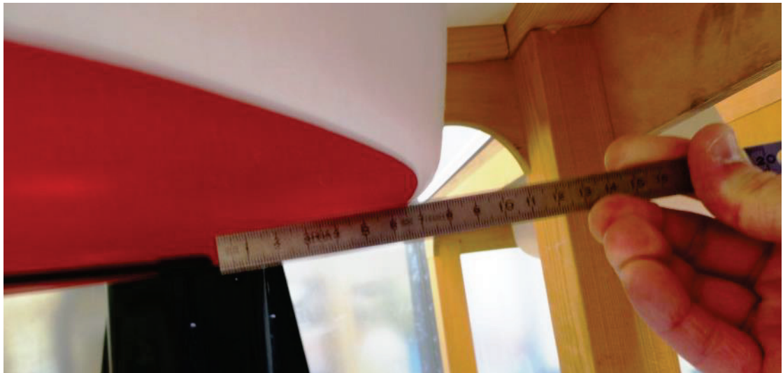
Fig. 14: NEARSON antenna, rear side at 0 mm from the phantom
