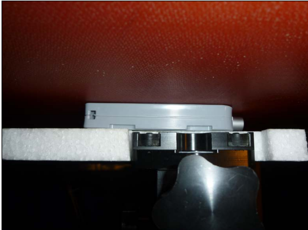
Fig. 8: Integrated Antenna, rear side at 0cm from the phantom
