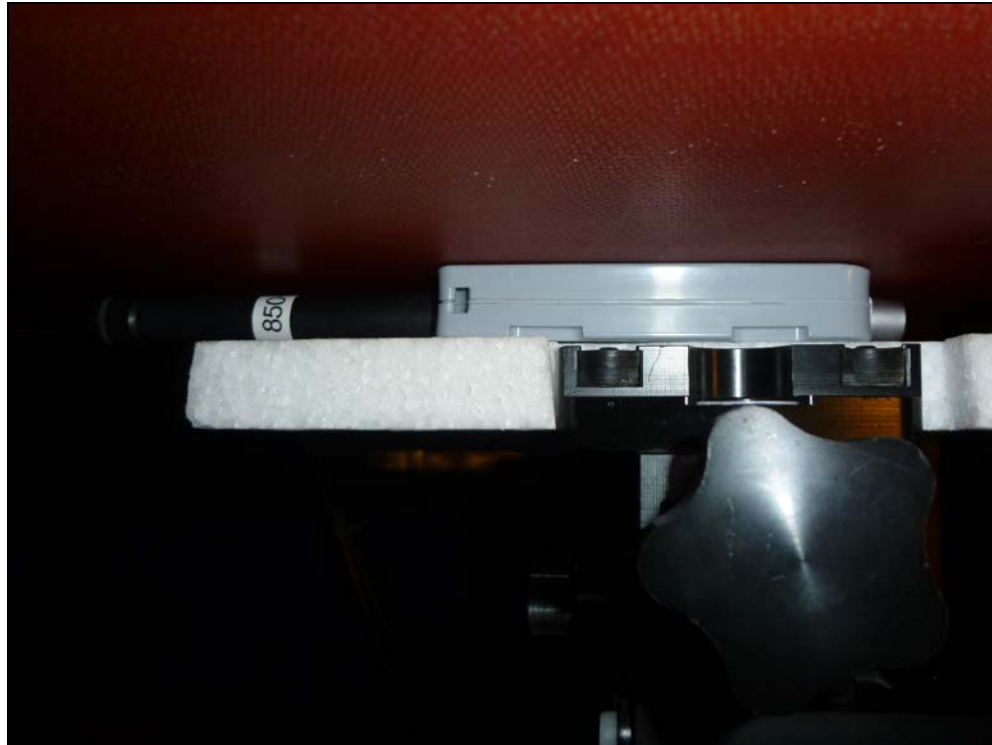
Fig. 11: External Antenna 2.0dBi, rear side at 0cm from the phantom
