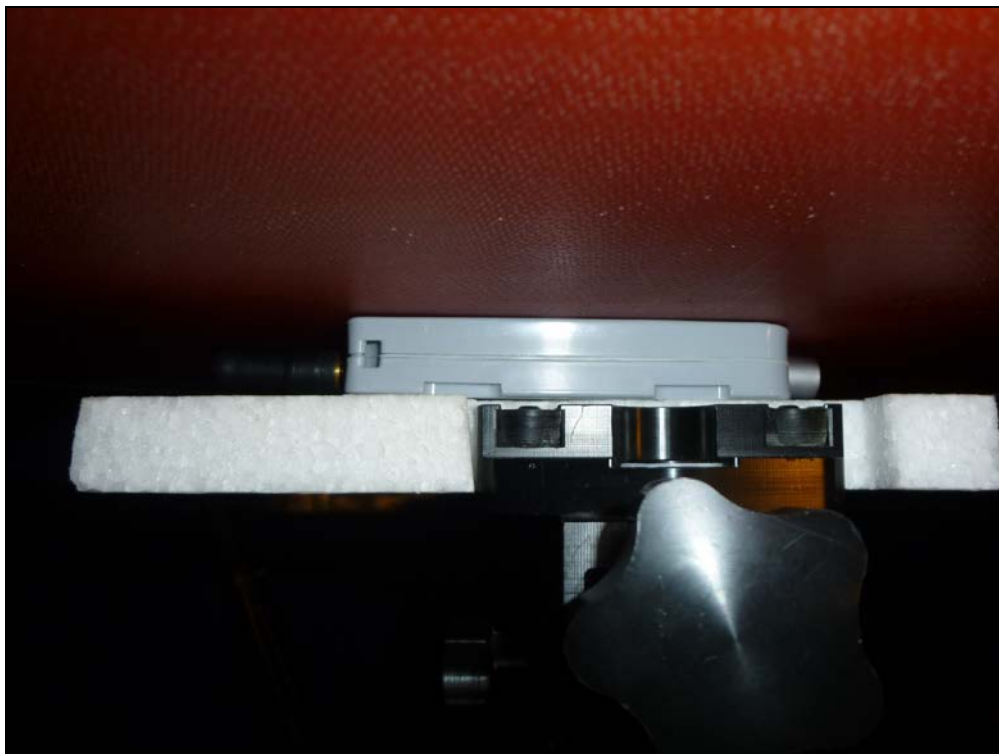
Fig. 9: External Antenna 0dB i , rear side at 0cm from the phantom
