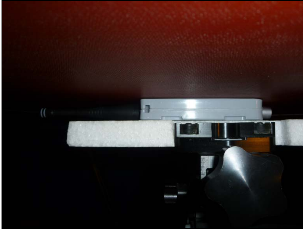
Fig. 10: External Antenna 1.8dBi, rear side at 0cm from the phantom
