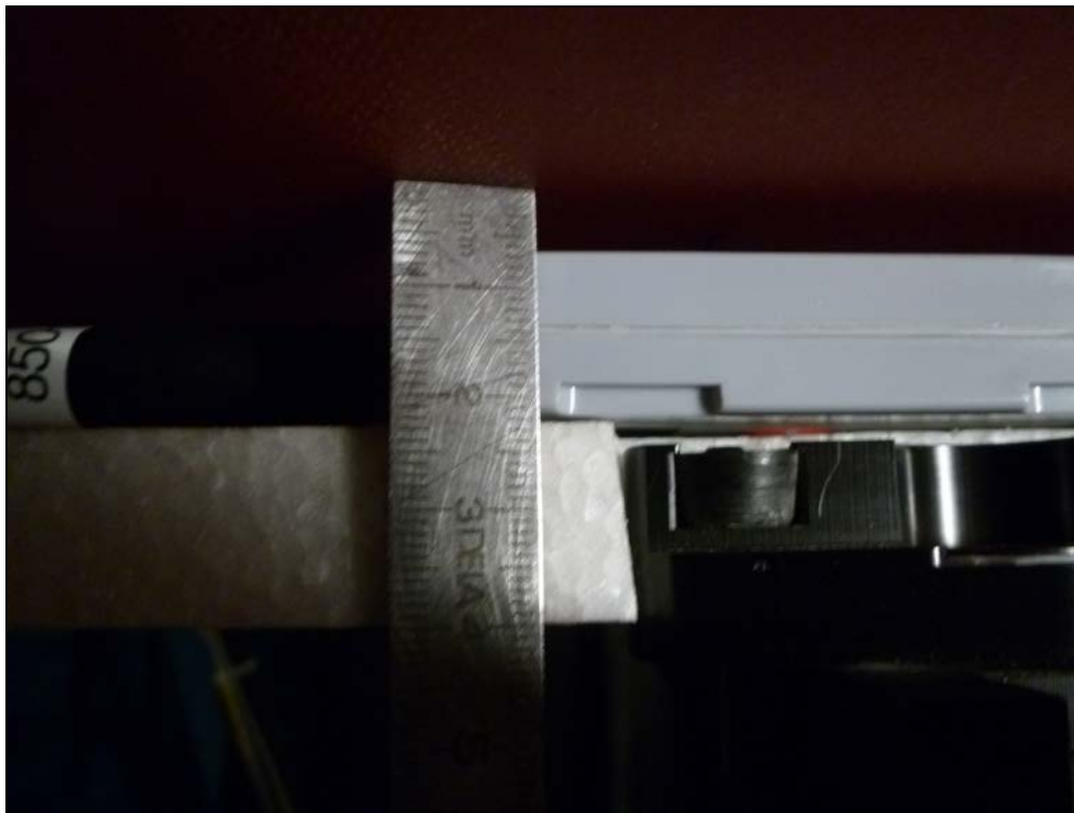
Fig. 12: External Antenna 2.0dBi, rear side at 0.5cm from the phantom
