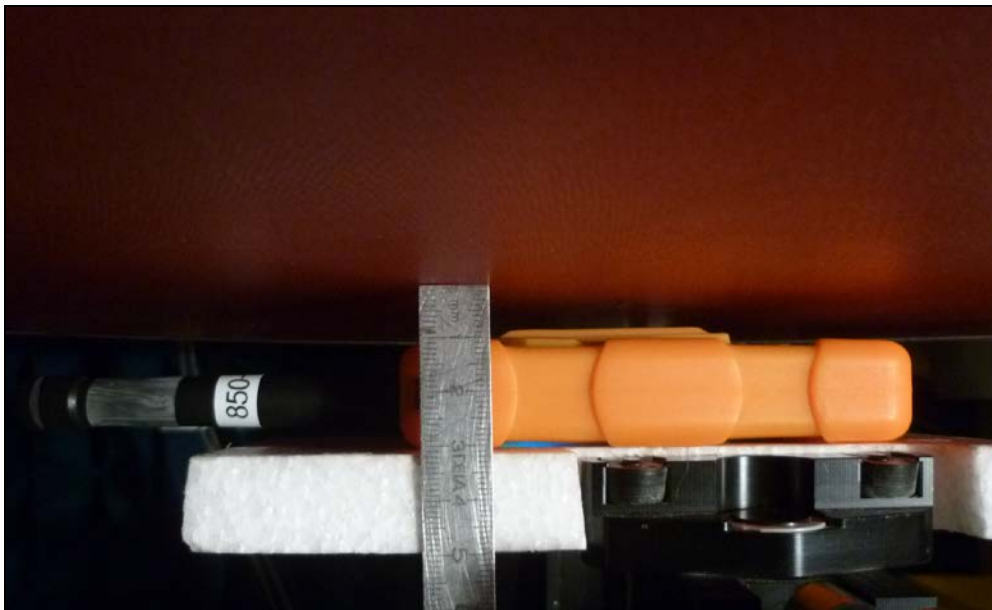
Fig. 13: External Antenna 2.0dBi, rear side with the rubber cover at 0.5cm from the phantom
