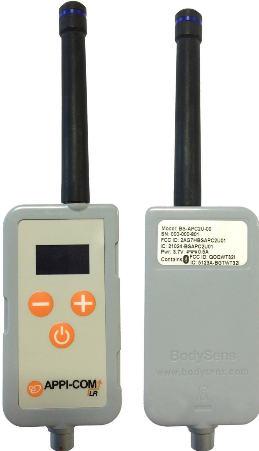
Figure 1. APPI COM LR Devices – similar to original APPI COM. Module with 1/2-wave antenna front and back with product label.
