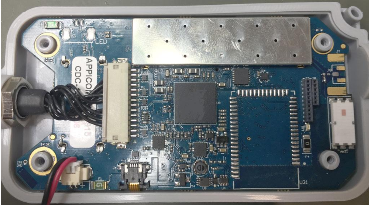
APPI COM LR MOUNTED INSIDE CASE WITH SHIELD AND CABLE ASSEMBLY
