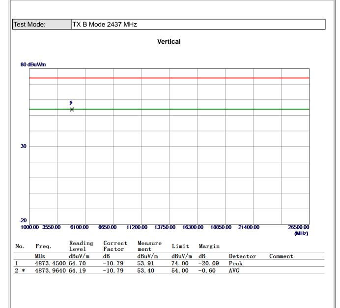
(1) Measurement Value = Reading Level + Correct Factor.
