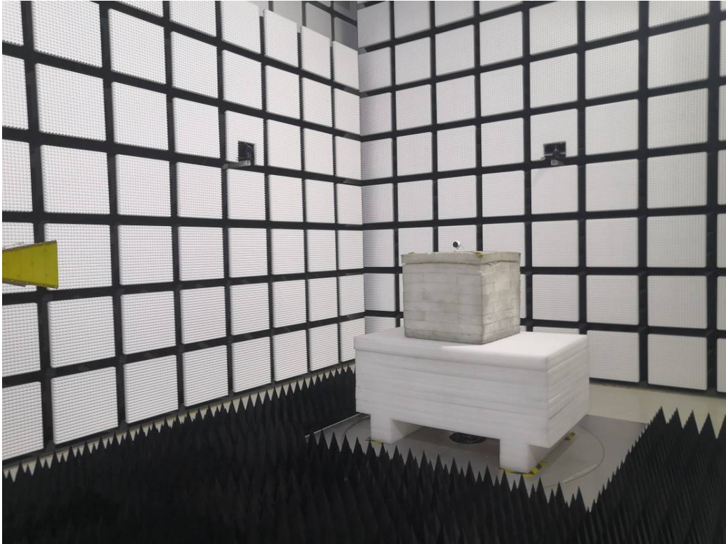
Radiated Emissions Above 1G front View -Mini 12S- Adapter 1#
