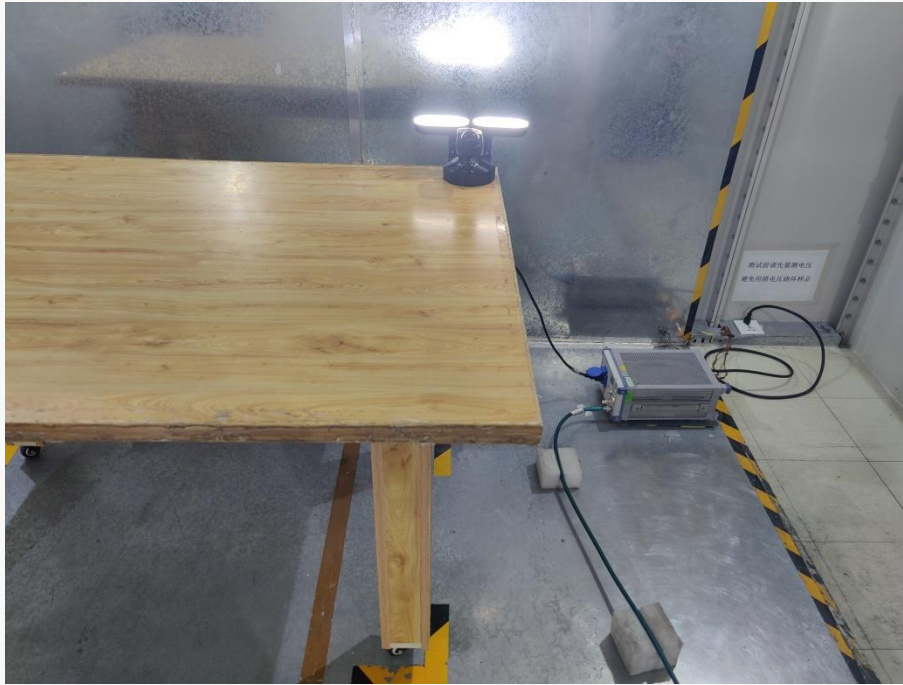
Conducted Emissions (Side View)
