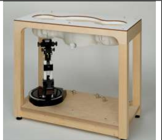
Fig. 8.7 Photo of SAM Twin Phantom
