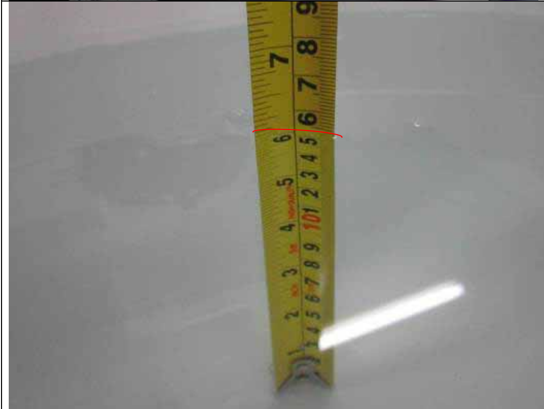
Liquid depth \geq 15cm
