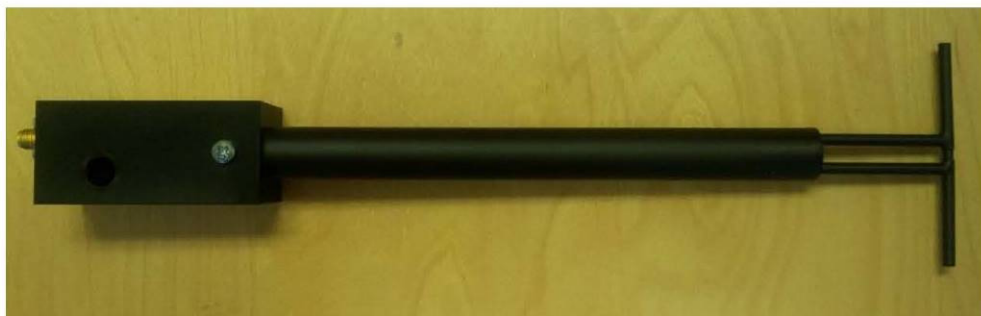
Figure 1 – MVG COMOSAR Validation Dipole
