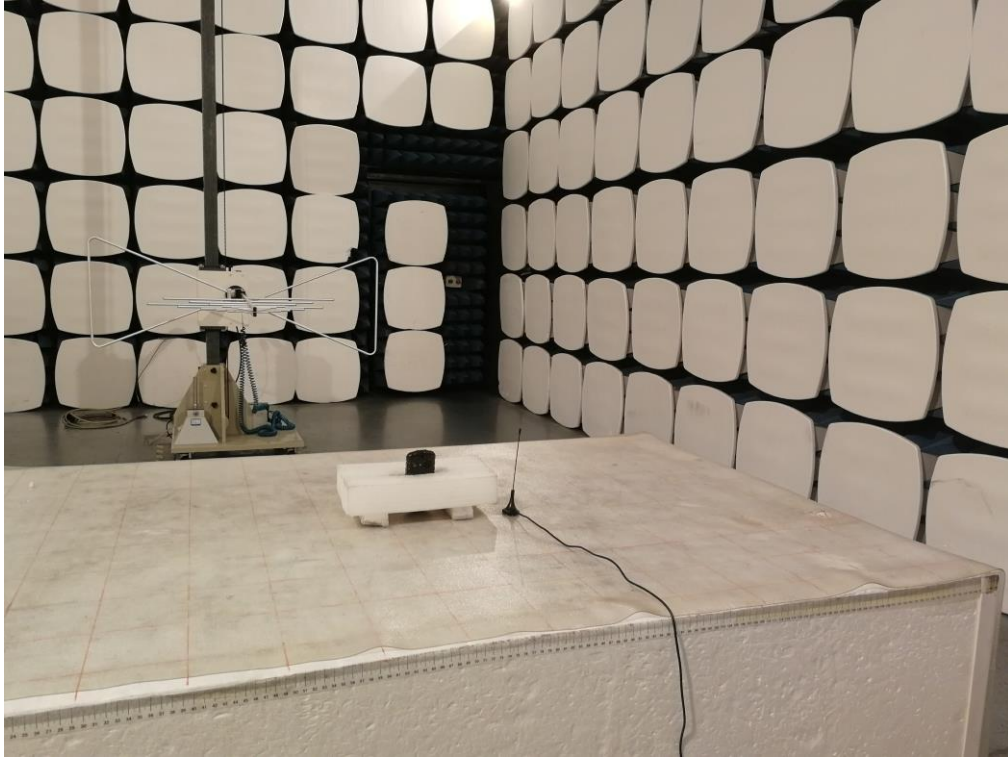
Radiated Spurious Emission Below 1GHz
