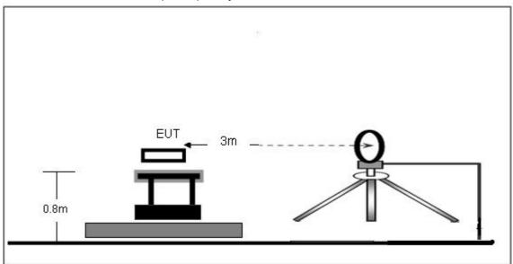
(B) Radiated Emission Test-Up Frequency 30MHz~1GHz
