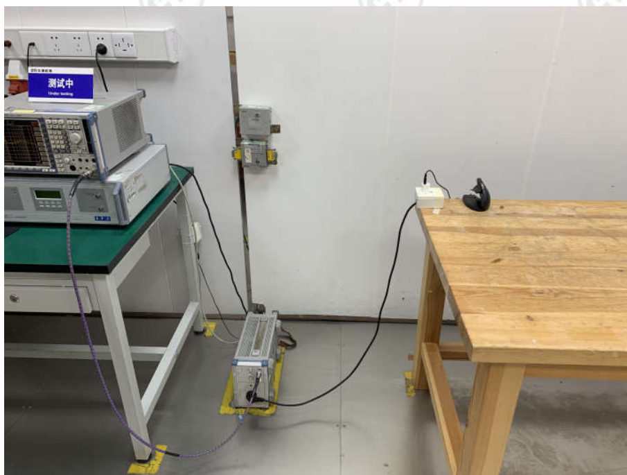
Conducted Emissions Test Setup
