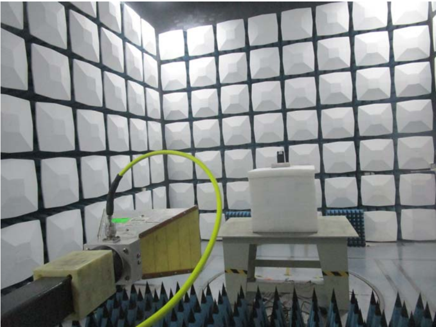
Radiated Emission Above 1GHz View
