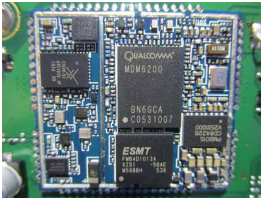
EUT- UMTS Module Uncover View
