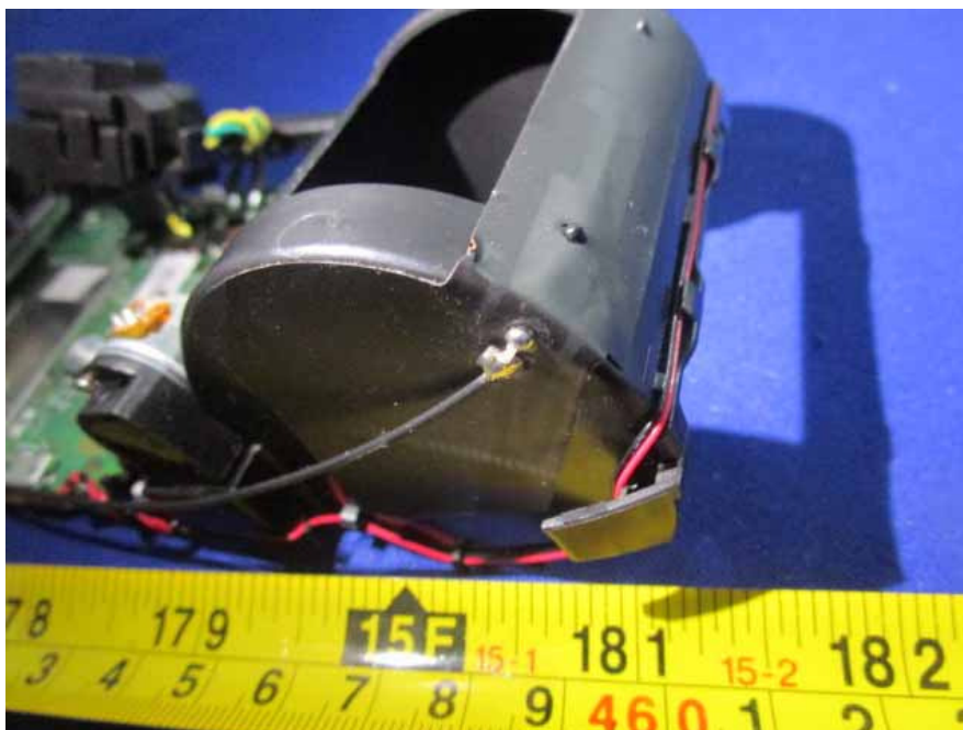
EUT- UMTS Antenna View
