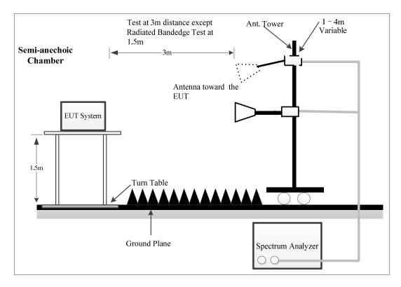
The radiated emission tests were performed in the semi-anechoic chamber, using the setup accordance with the ANSI C63.10-2013. The specification used was FCC 15.209, FCC 15.407, RSS-247, RSS-Gen limits.
