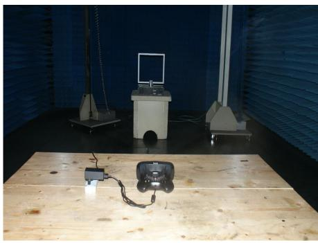
Photograph 2: Set-up for Radiated Spurious Emission, 30MHz - 1GHz
