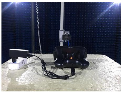
Photograph 4: Set-up for Radiated Spurious Emission, 18GHz - 26.5GHz
