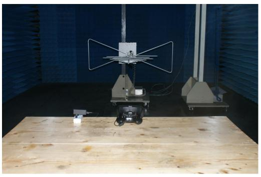
Photograph 6: Set-up for Radiated Emission, above 1GHz
