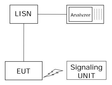
Setup in the shielded room for conducted measurements at AC mains port
