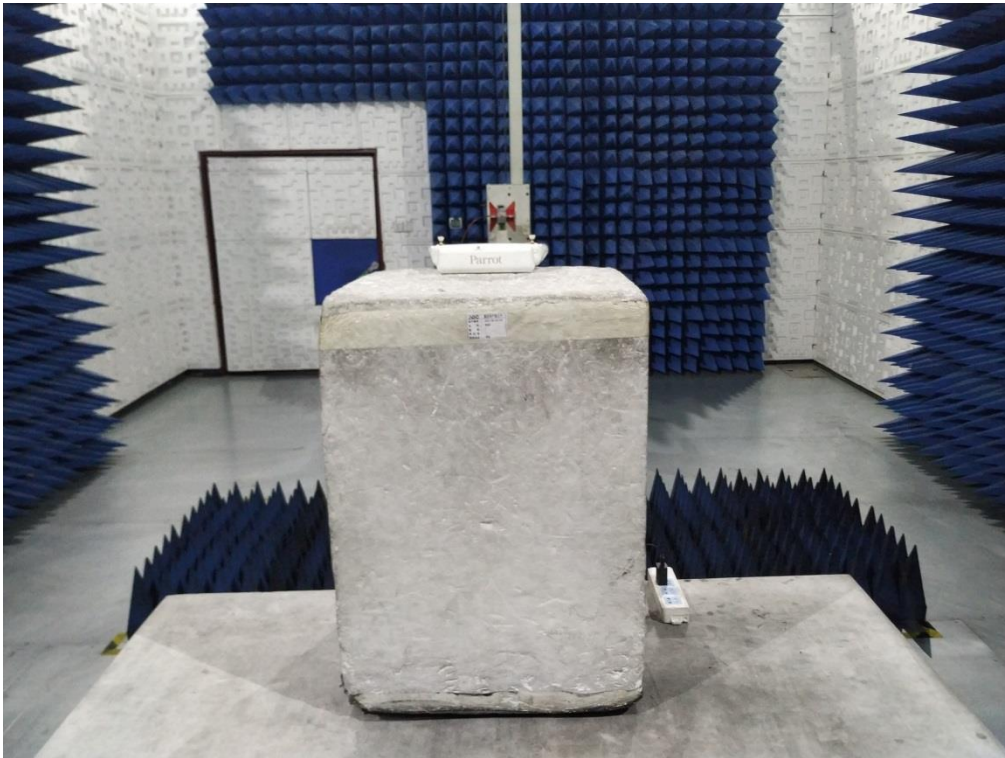
FCC RADIATED EMISSION TEST SETUP ABOVE 1GHZ
