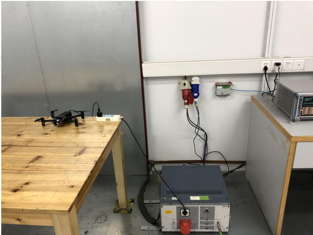
FCC RADIATED EMISSION TEST SETUP BELOW 1GHZ
