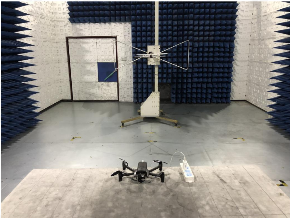
FCC RADIATED EMISSION TEST SETUP BELOW 1GHZ
