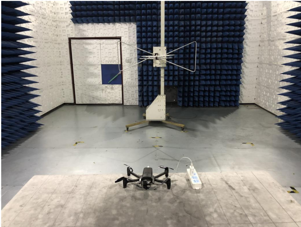
FCC RADIATED EMISSION TEST SETUP ABOVE 1GHZ
