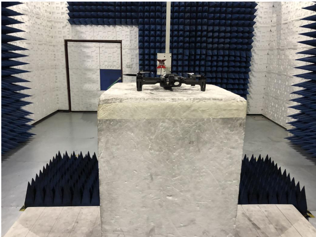
FCC RADIATED EMISSION TEST SETUP ABOVE 1GHZ
