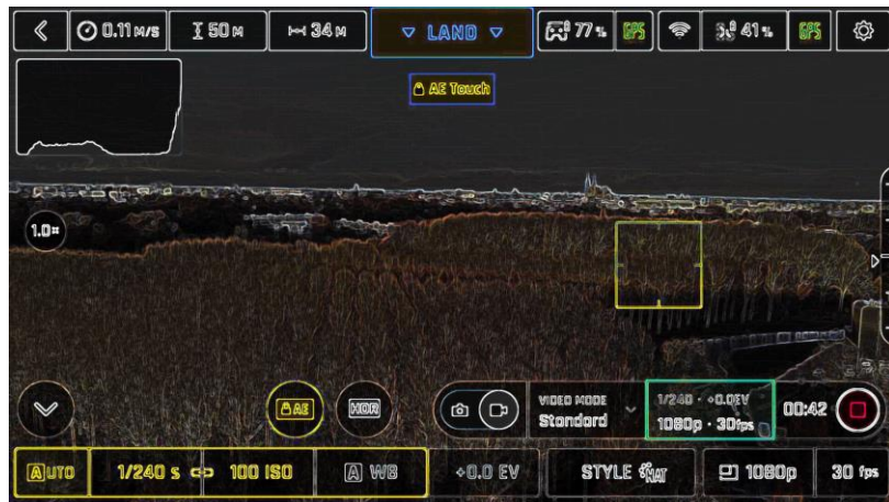
Exposure is locked on the top of the trees: shutter speed is set at 1/240 s
