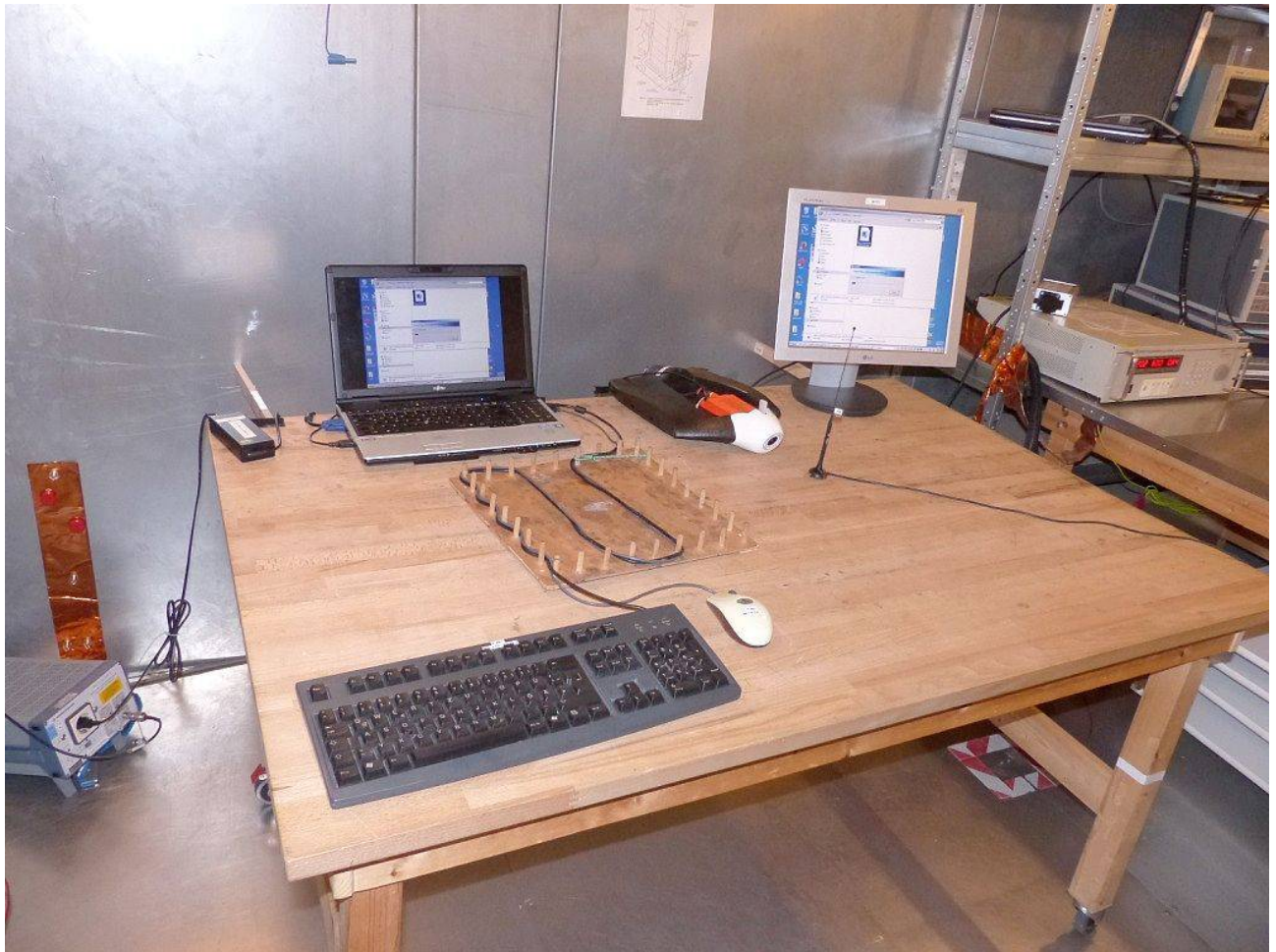
Photo 5: Test setup for conducted measurements (computer peripheral setup, EUT connected by USB-cable to computer, unintentional radiator §15.107, ANSI C63.4)
