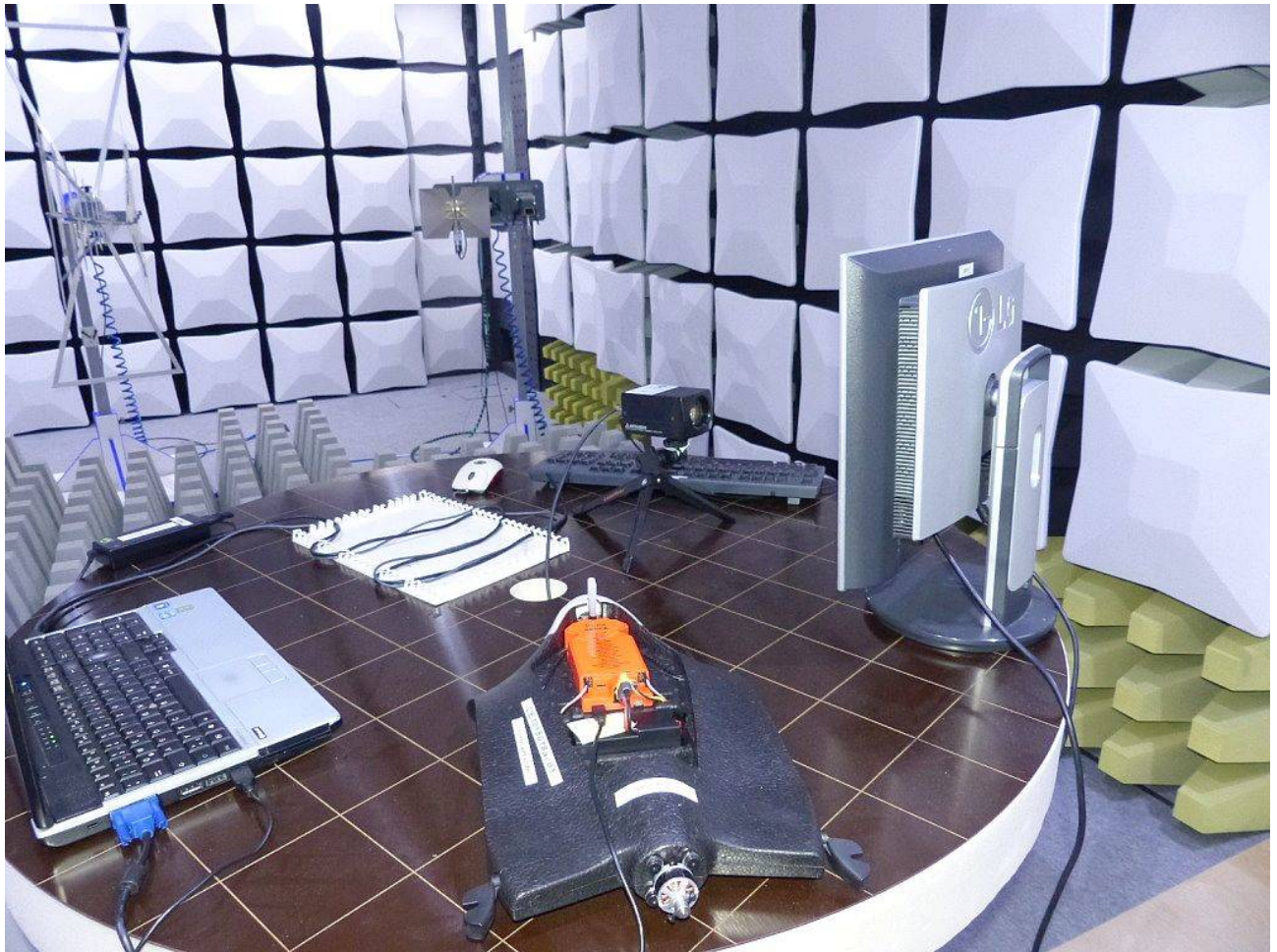
Photo 9: Test setup for radiated measurements (computer peripheral setup, EUT connected by USB-cable to computer, unintentional radiator §15.109, ANSI C63.4, in Fully-Anechoic Chamber, 1 – 4 GHz)
