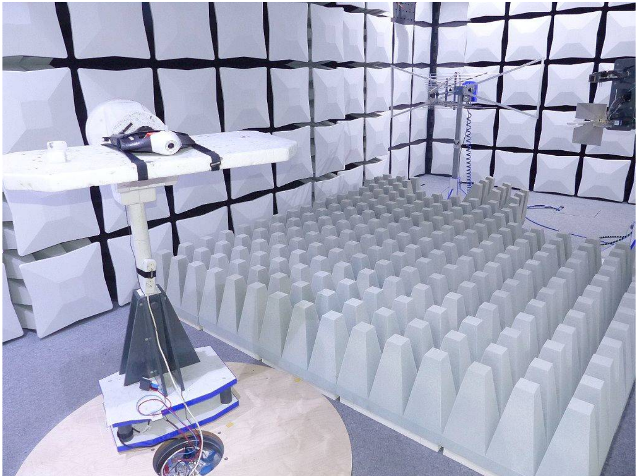
Photo 3: Test setup for radiated measurements (Enclosure, fully-anechoic chamber, 1 – 26.5 GHz intentional radiator §15, ANSI C63.10)
