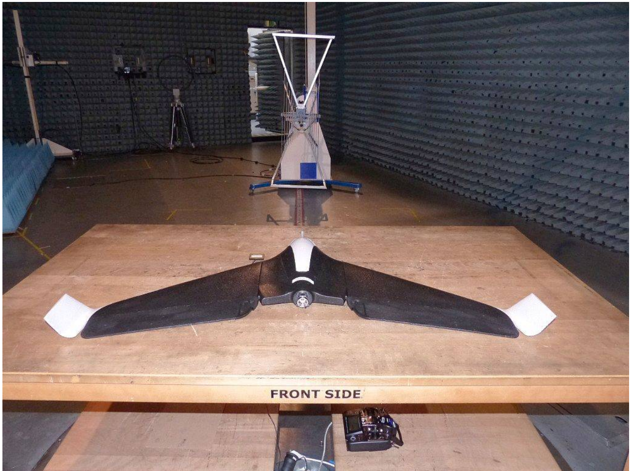
Photo 6: Test setup for radiated measurements (EUT connected to auxiliary 2.4 GHz remote control receiver, unintentional radiator §15.109, ANSI C63.4, in Semi-Anechoic Chamber, 30 MHz – 1 GHz)
