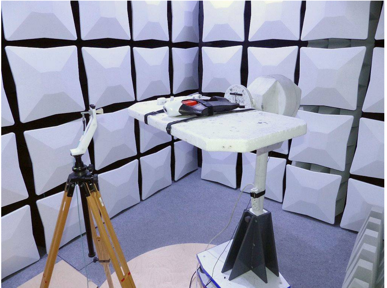
Photo 4: Test setup for radiated measurements (Enclosure, fully-anechoic chamber, 26.5 – 40 GHz intentional radiator §15, ANSI C63.10)
