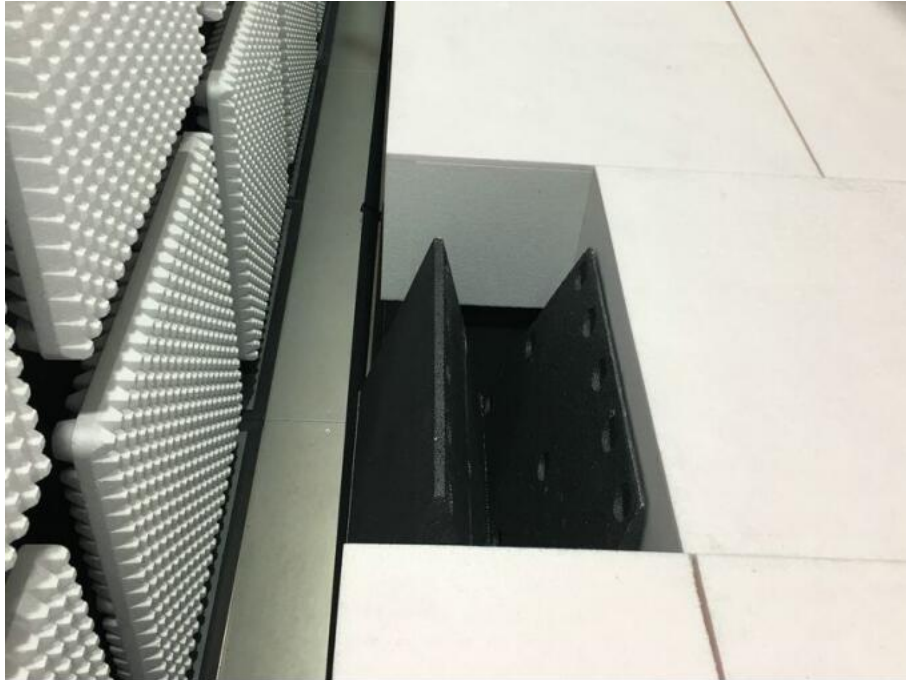
Radiated spurious emission Test Setup-3 There are absorbing materials under the ground.
