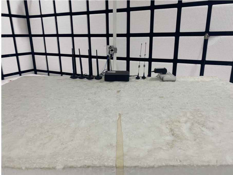
Radiated spurious emission Test Setup-2(Above 18GHz)
