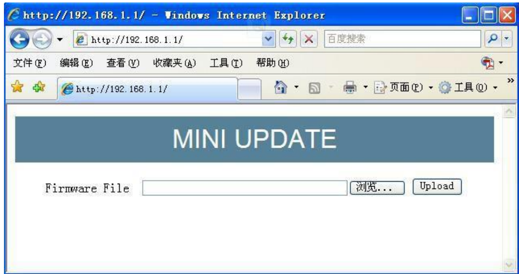
Figure 5-72 CFE mode upgrading
