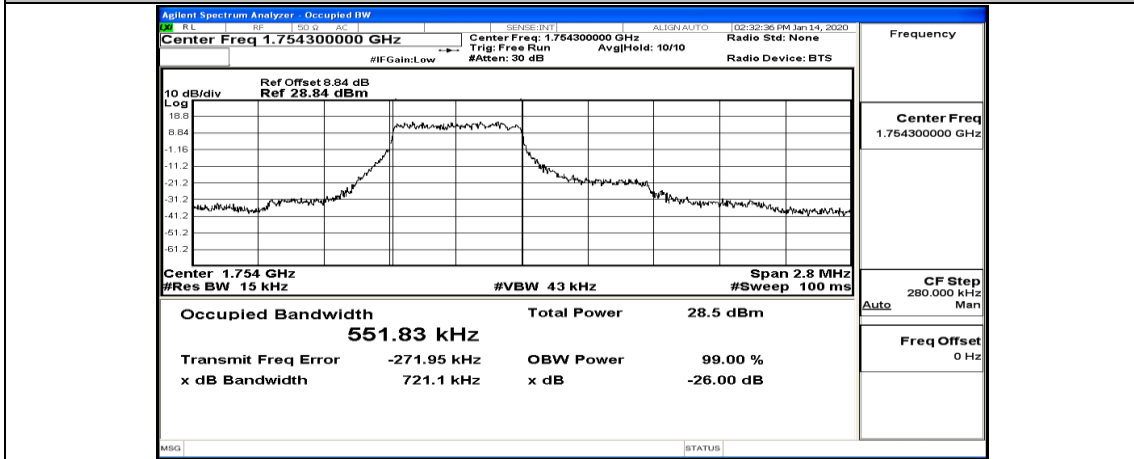
(Channel Bandwidth: 1.4 MHz)_HCH_QPSK_3RB#2
