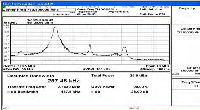
(Channel Bandwidth: 5 MHz)_LCH_16QAM_1RB#12
