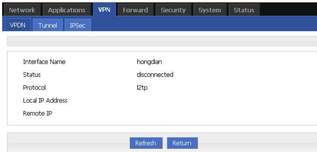
Figure 5-58 L2TP tunnel status
