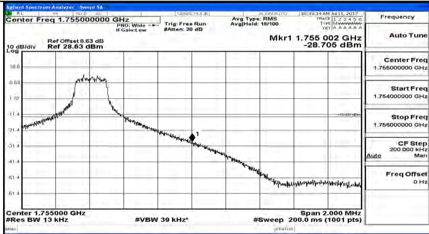
Channel Bandwidth: 10 MHz_HCH_16QAM_25RB#0
