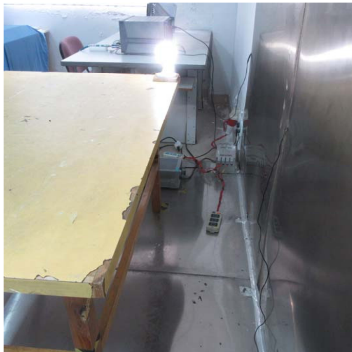
Conducted Disturbance Test Setup Side View
