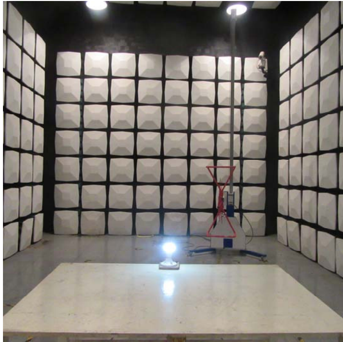
Radiated Disturbance Test Setup Rear View (Below 1GHz)
