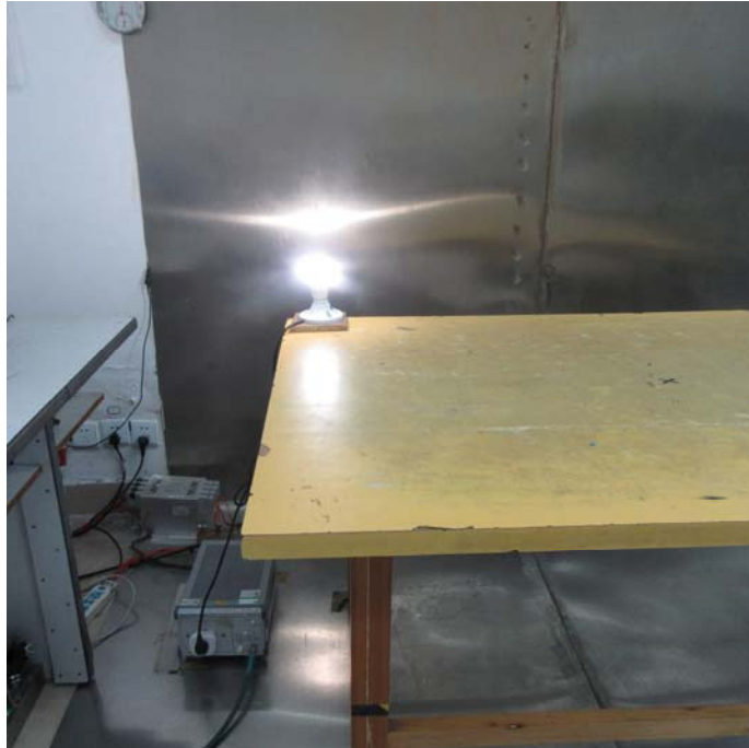
Conducted Disturbance Test Setup Front View
