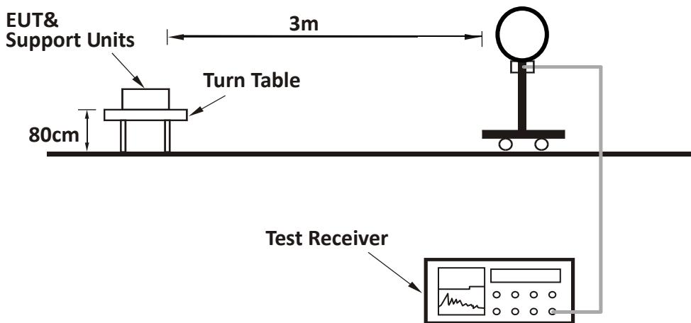
**For Radiated emission 30MHz to 1GHz:**
