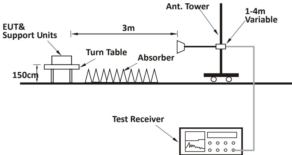
**TEST REPORT****7.4 Test Results of Radiated Emissions**
