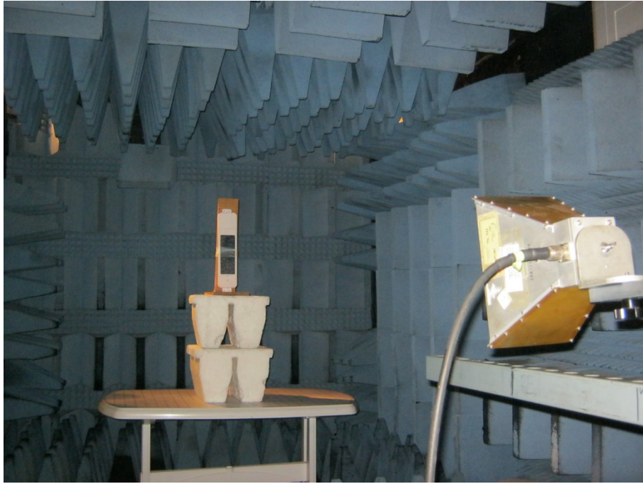
Radiated Emission Test, 1-18GHz and Intermodulation Radiated Emission Test
