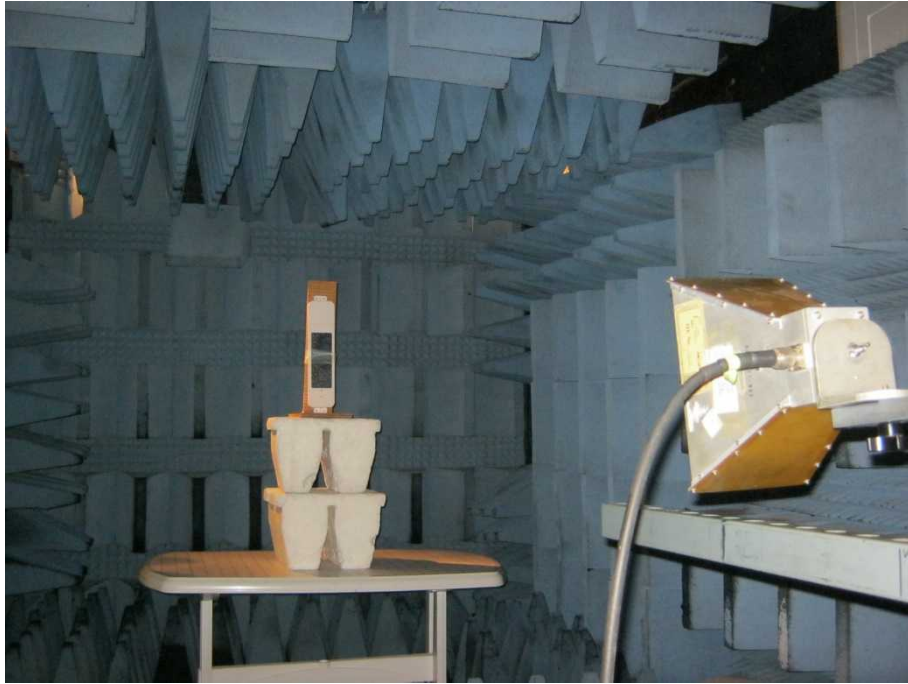
Figure 8. Radiated Emission Test, 1-18GHz and Intermodulation Radiated Emission Test
