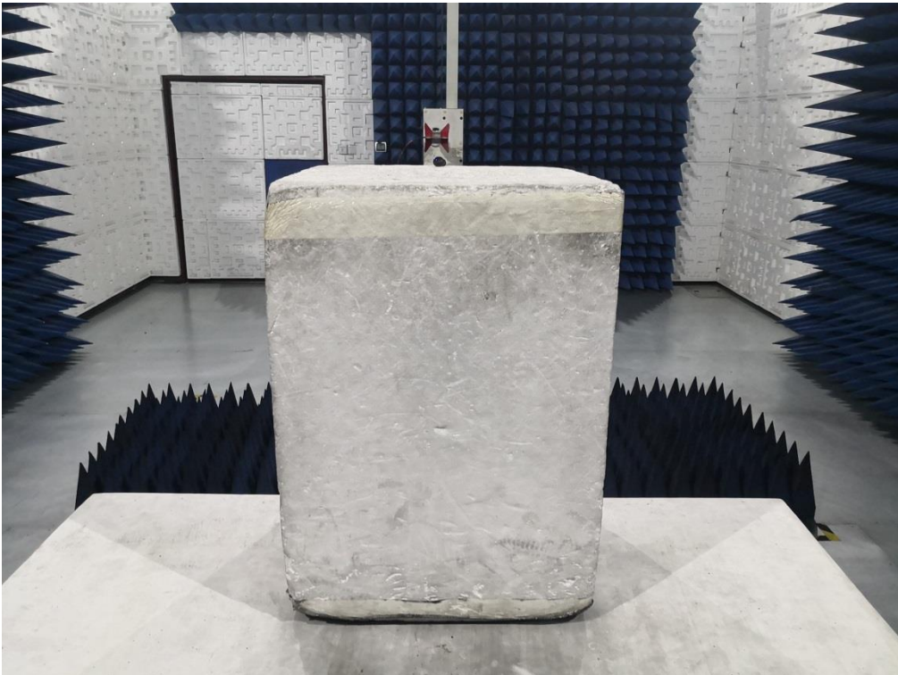
RADIATED EMISSION TEST SETUP ABOVE 1GHz
