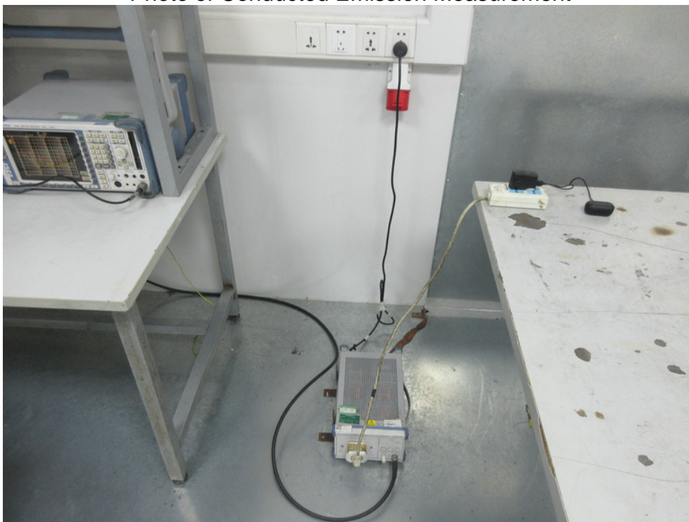
FCC ID: 2AG68-TWS824A Photo of Conducted Emission Measurement
