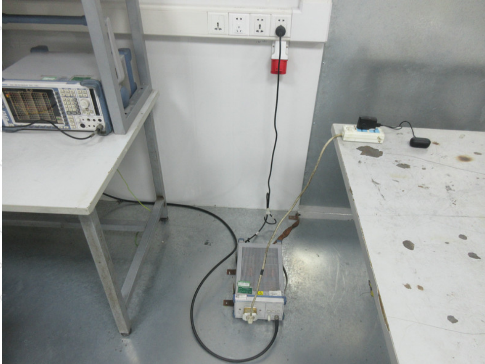
Photo of Conducted Emission Measurement
