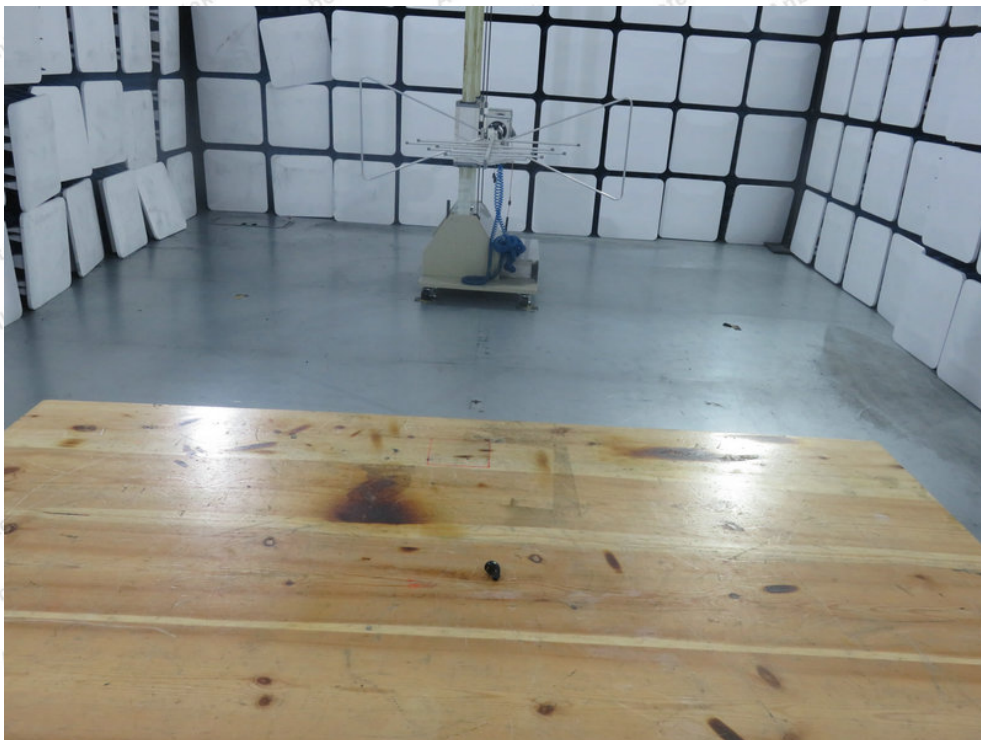
Photo of Radiation Emission Test
